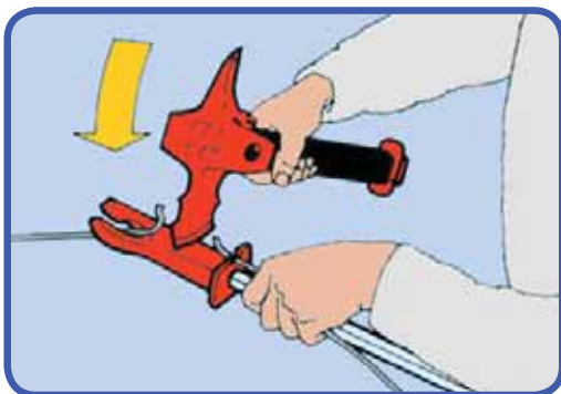
5. Wire, ropes, cables etc. - short hits - support rod against arm.
