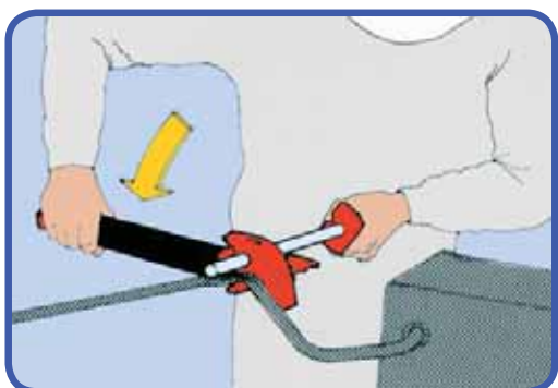
3. Flattening pipe - stopping liquid flow.
