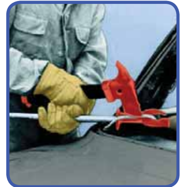
3. Cut cables while holding them with claw apart.
