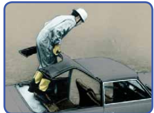
7. Fold the roof open.
