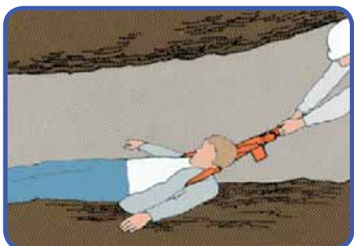
3. Pulling with belt - twisted belt gives head support.
