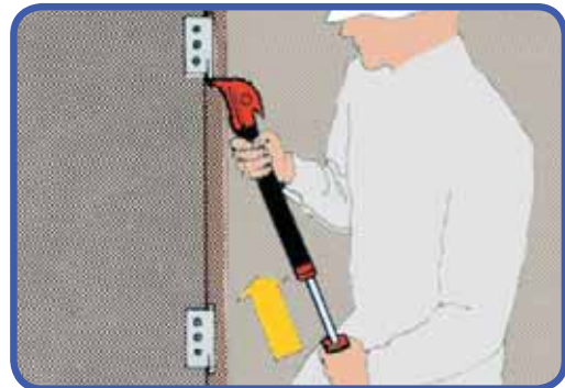
4. Pushing in pins, dowels etc.
