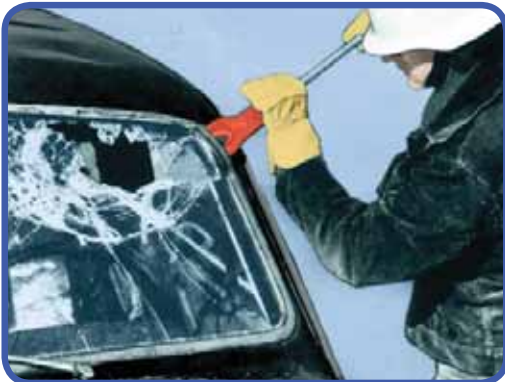
3. Loosen rubber insert with chisel.
