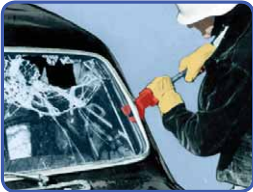
1. Loosen chrome strip with chisel or axe-pick.
