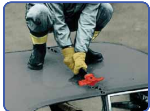
5. Break the roof with a few strong blows.
