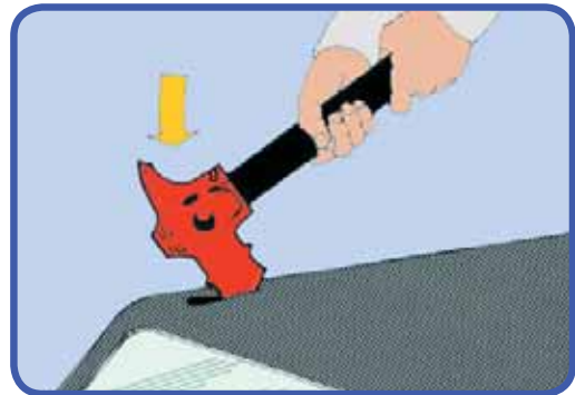
6. Car roof, etc. - slanting short hits.
