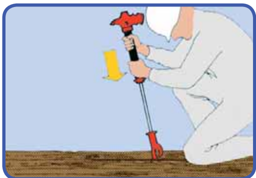
1. Pierce floor with pumping motion.
