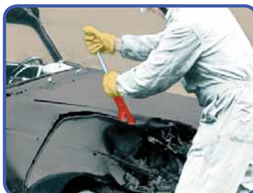
4. Cut the mudguard - use the claw part.
