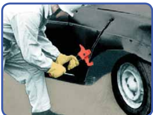
3. Cut the mudguard - use the edge.
