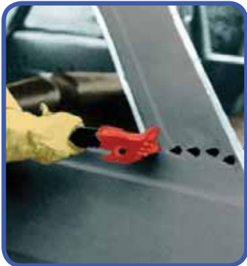
1. Perforate the lower part of the roof pillars with the pick.
