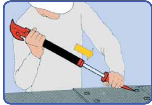
2. Cutting off rivet- and boltheads.
