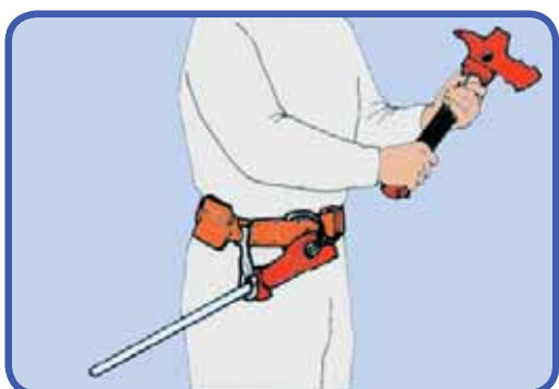
7. Claw part attached to hook and D-ring.
