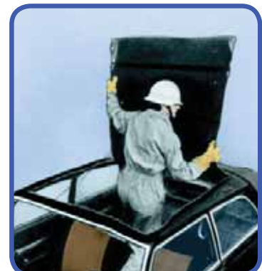
6. Fold the roof back.
