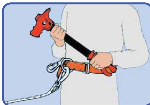
6. Belt used as safety belt.
