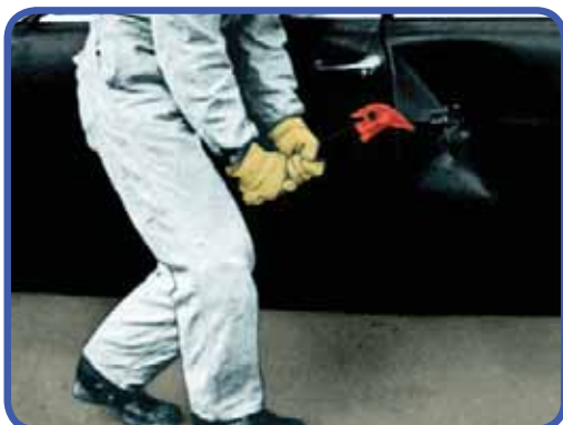
5. Turn upwards. The door is lifted - structure is bent apart - opening of the door increases.
