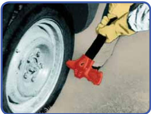
3. Puncture tyres with the pick - hit close to rim.
