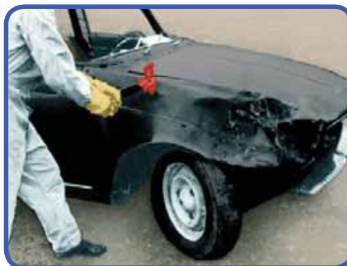
2. Cut the mudguard - use the pike.
