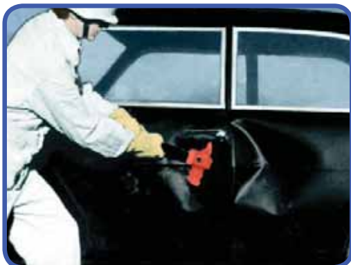
3. Hit on both sides of the lock.
