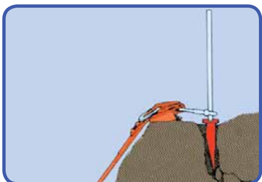
3. Anchoring in rock - claw part well inserted.
