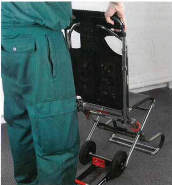
Figure 16 - Preparing to attach Track to unoccupied Chair
